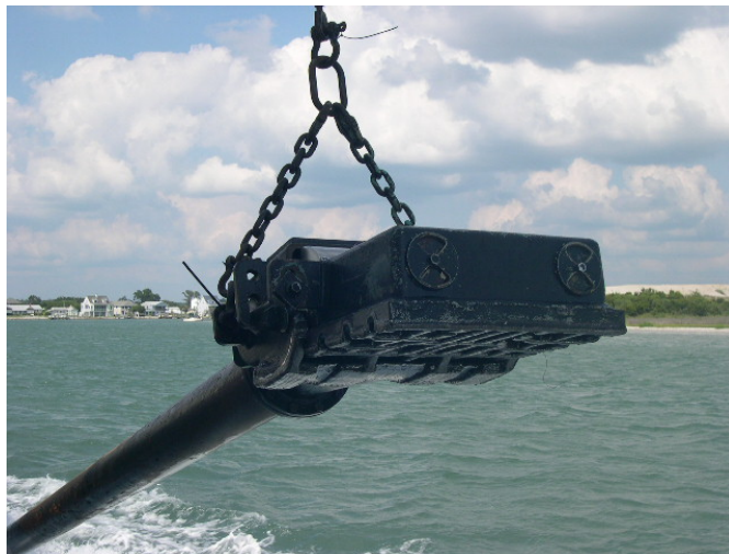
The Fry's draghead, the workhorse that maintains many of the waterways comprising the "Southern Inlet System".
