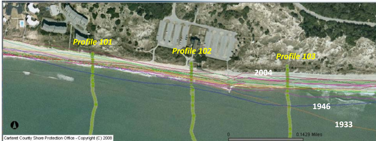
Fig. 2 – A 2004 aerial photograph at the bath house, Ft. Macon State Park. Three of the County's profiles are positioned and labeled in the photograph in addition to multiple shorelines that have been traced using the wet/dry method described in this article (only the 1933, 1946, & 2004 pictures are labeled).
