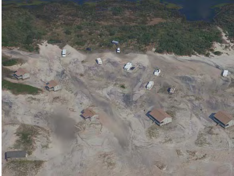
Fig. 5 – Aerial photograph depicting overwash sand impacting cabins and RVs at south Core Banks, Cape Lookout National Seashore.
